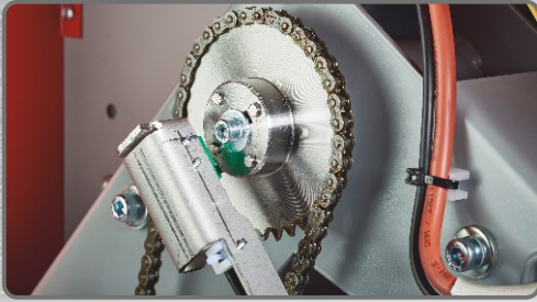
Secure rotation monitoring with dust insensitive magnets.
